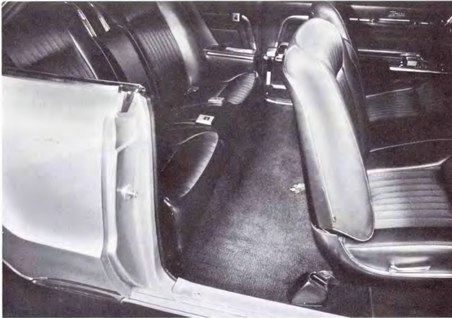
Fig. 3—WIDE DOOR DESIGN, STRATO SEATS. To provide easier access to the rear seat, the Toronado features a door that is 3.5 in. wider than comparable coupe doors. This provides a 37-in. wide opening to the passenger compartment when fully opened. Six passengers may sit comfortably in the newly designed front and rear seats. In the standard Toronado model, a conventional bench seat is used, while in the deluxe model a specially designed strato bench seat (shown here) is standard equipment. Available as optional equipment on the strato seat is an infinitely adjustable reclining right side front passenger seat, which may be tilted rearward to a maximum of 30° from the normal position. Adjustable headrests are available for the driver and passenger on all front seats.
