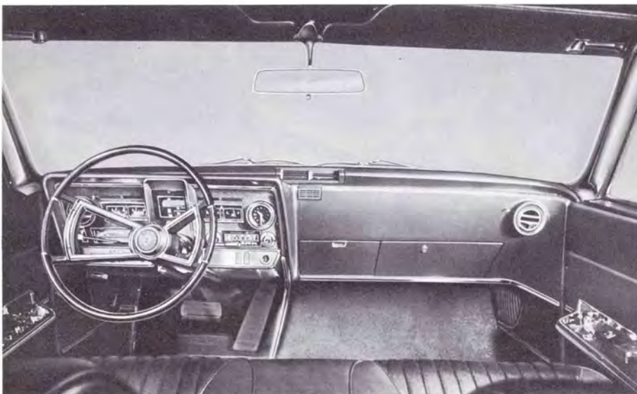
Fig. 4—INSTRUMENT PANEL DESIGN. All controls and instruments are mounted in one die casting located directly in front of the driver. Instruments include needle type ammeter and temperature gages. The speedometer is a drum dial type. The padded instrument panel extends the full width of the car.
