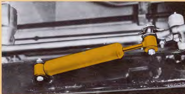
Fig. 11—STEERING SYSTEM. Power steering is standard equipment on the Toronado. The steering system includes a shock absorber connection (bottom) between the linkage and the vehicle frame.
