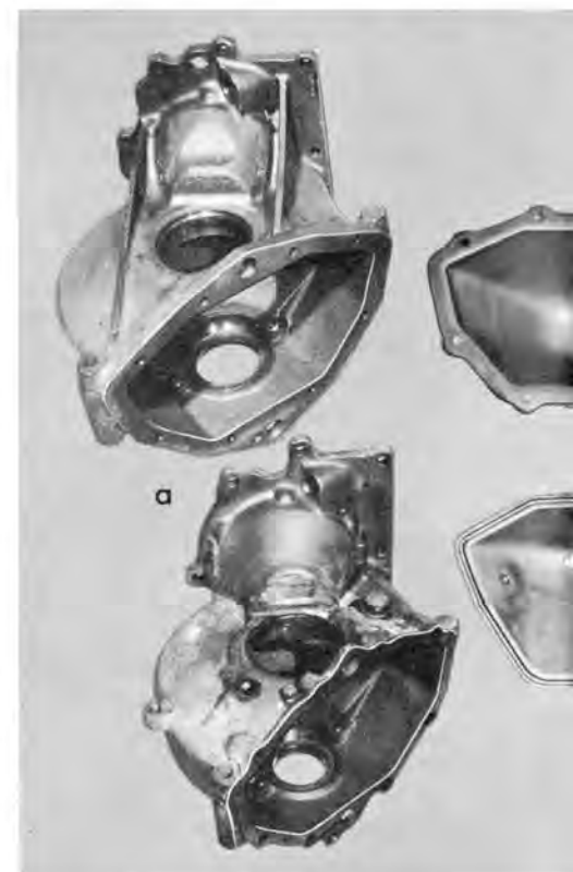
Fig. 7—COMPARISON OF VARIOUS FINAL DRIVE COMPONENT DESIGN CHANGES—EXPERIMENTAL AND PRODUCTION. During the development of the final drive for the Tornado, various components went through design changes as the system evolved through its experimental stages to the production version. Shown here are some of the components and the changes between the experimental design (top) and the production design version (bottom). The components are: differential carrier housing (a), differential cover (b), ring gear and drive pinion (c), differential case cover (d), differential gear case (e), and planet pinion gear (f).
