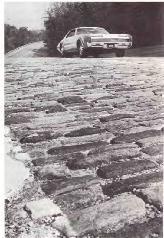
Fig. 7—BELGIAN BLOCK ROAD. This road at the GM Proving Ground is constructed of rectangular stone blocks laid in an uneven pattern to form a road surface. The contour of the road provides various turns and dips. The Belgian block test schedule provides accelerated testing of structural items such as body, frame, and all suspension components. The severity of the course is such that low test mileage often is sufficient to prove the durability of components on test.
