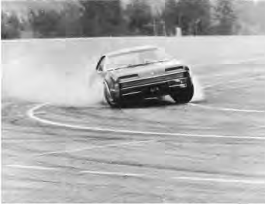
Fig. 8—J-TURN TEST. During a J-turn test, such as the one shown here being conducted at the GM Proving Ground, both the driving and turning forces are absorbed in the front suspension. The car undergoing a J-turn test is driven at approximately 50 mph, then is placed quickly into a locked turn with power maintained.
