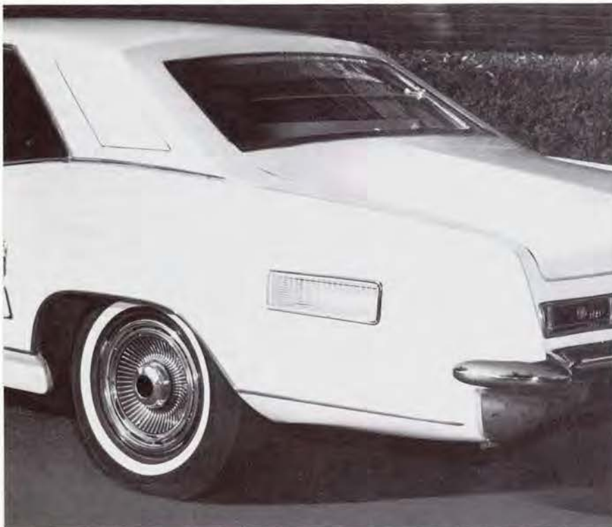
Fig. 6—REAR QUARTER PANEL VENTS. Another possible location for the extractor was the rear quarter panel. This location was investigated by modifying a car with a flush extractor vent in the panel. Tests indicated that static air pressure at 60 mph in this location was -0.009 psi (relative to atmospheric pressure).
