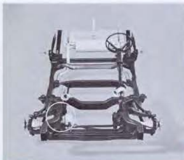
Fig. 5—STEERING COLUMN ANGLE. A universal joint added to the steering column provides the Toronado with a comfortable steering column angle.
