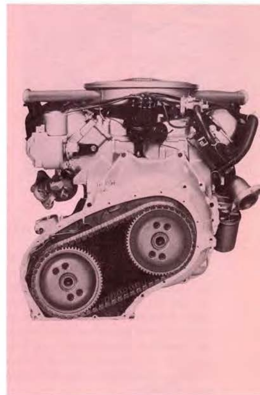
Fig. 9—TRANSMISSION DRIVE CHAIN AND SPROCKETS. The Toronado transmission is split between the torque converter, which is attached to the rear of the engine, and the mechanical transmission, which is attached to the differential. These two sections of the transmission are connected by a chain and sprocket system to form the transmission assembly. The photograph shows a rear view of the transmission-engine unit with the chain cover removed.
