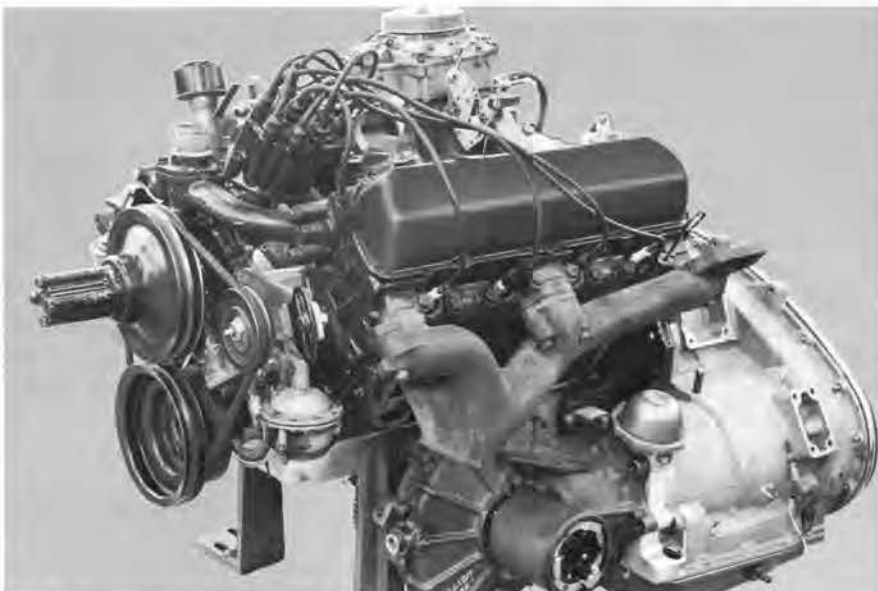
Fig. 2—PROTOTYPE UNITIZED POWER PACKAGE. A 429-cu in. engine was used for the prototype UPP developed by the GM Engineering Staff. This was the largest engine available for application in the UPP vehicle. Front end mounting locations for the distributor and oil pump permitted a greater degree of flexibility at the rear of the engine for mating with the automatic transmission.
