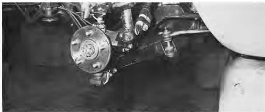
Fig. 1—DYNAMIC STEERING TEST INSTRUMENTATION. Multiple needle recording and plotting instruments (top) mounted in the rear seat of the test car were used in the dynamic testing of front suspension components (bottom). Wheel angularity and joint forces were measured in tests of this type.
