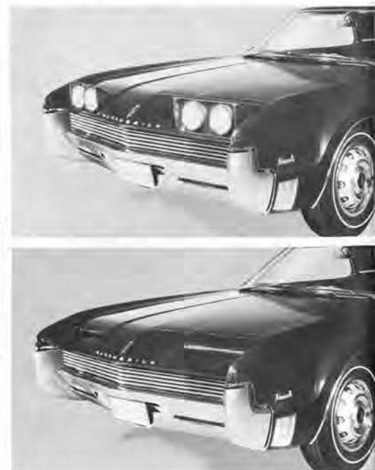
Fig. 11—HEADLAMP ACTUATOR. Vacuum power cylinders actuate the Toronado headlamp assembly through pistons connected to linkages. The headlamps are raised into position when the headlamp switch is turned on and lower when the switch is turned off.
