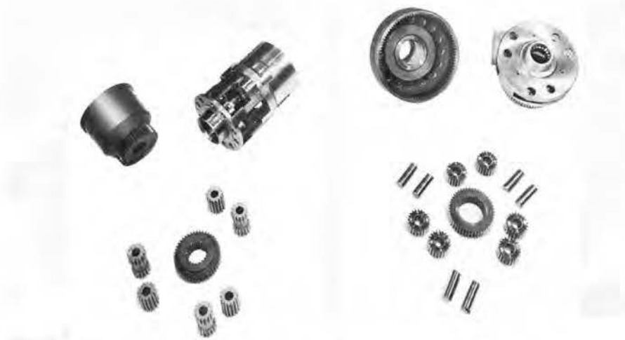
Fig. 7—PLANETARY DIFFERENTIALS. Shown here are the two types of planetary differentials tested in the pre-production UPP design. The design at the left, a radially compact unit, had a carrier input and sun gear outputs to each wheel. The design at the right, and the one eventually selected for the production design, had a ring gear input with a sun gear and carrier output.
