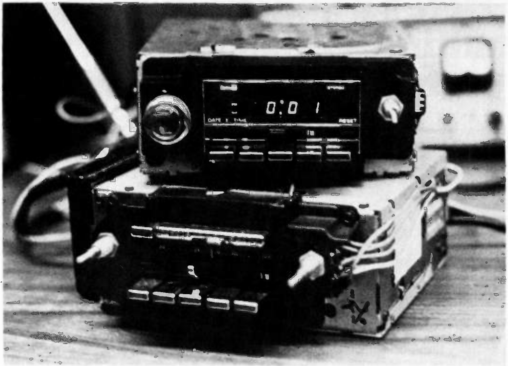
Fig. 1—The 1977 Delco digital AM/FM radio and FM stereo unit shown in the elapsed-time-mode.
